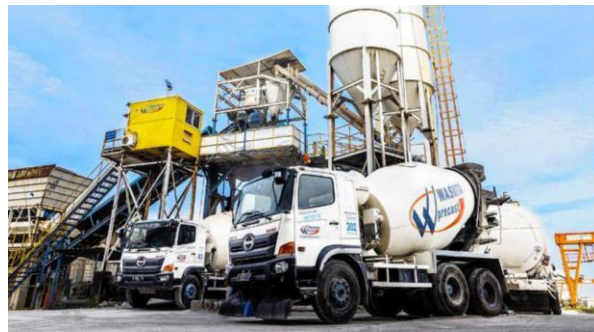
Figure 3. Photograph of the Self-Managed Batching Plant at the Musi V Bridge Project
