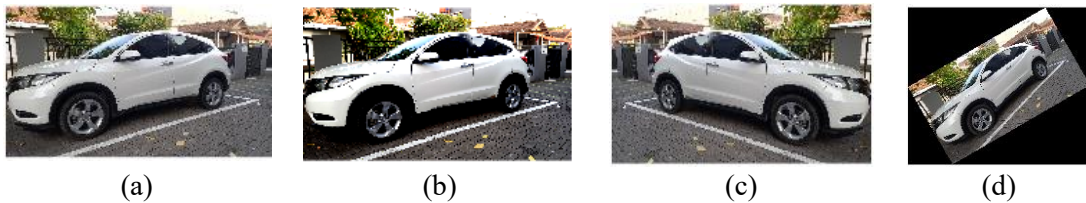
Figure 3. Example of the results of the Data Augmentation process: (a) original image, (b) brightness adjustment, (c) flip horizontal, (d) rotation using 30°
